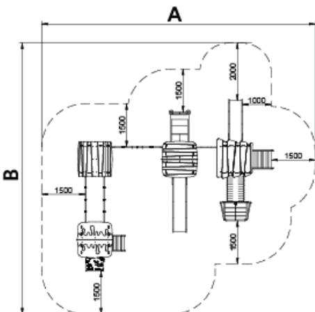
Playground collection **made with maintenance-free materials**: mixed extrusion post made of aluminum and polymer, one-piece aluminum steps and the anti-slip polymer platforms. The user will find inclusive games in every part of the structure.
