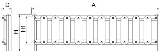
**Structure, Laminated wood:** scandinavian laminated pine wood treated in autoclave Class IV. Finished with two layers of Lasur paint. - In case of being subjected to bad weather conditions, laminated pine wood can present some tiny cracks on the surface that do not reduce its durability at all. As regards resin and knots, please note that these are part of its natural appearance.
