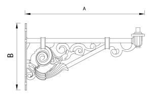
Classic bracket for column or wall mounting; (IRVI71) **made of recycled and recyclable plastic (REBNEW)** for Class II being a durable maintenance-free material, (IRVI71P) made of aluminium. Both options finished in black RAL 9005 and top fixing by means of a 3/4" fitting.
