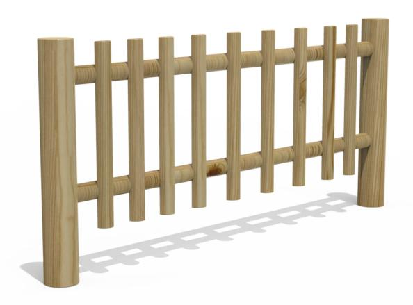
Fence made of pine wood reated in vacuum pressure autoclave Class IV against woodworm, termites and insects. Ø120 x 1500mm posts. Ø80 x 2000mm railings. Ø90mm semi-circulars bars.
