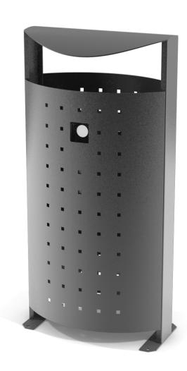
Zinc-plated steel inner bin and lid. Internal system with ring to fix the plastic bags, top lid and front door. Removable built-in ashtray. Epoxy coating and martele black polyester powder coating. Recommended anchoring: floor mounting by means of Ø10 screws, not supplied.
