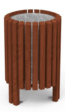
Litter bin made with inner and outer metal structure with twenty-four 40x35 tropical wood boards treated with Lignus, a fungicide, insecticide and waterproof agent. Mahogany colour finish. Galvanised steel inner bin.
